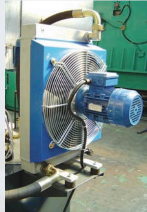
Air cooling system.
