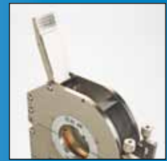
"Flip-top" hinges open for final inspection of tube alignment prior to welding.
